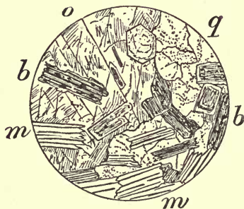
Fig. 24. — Granite. Near Dublin. \times 12 . b , Dark Mica, with deep brown patches included. m , Muscovite. Near the top of the field a hexagonal (basal) section occurs. o , Orthoclase. q , Quartz.
